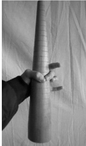
Figure 4 : Measuring grip span using a grip span cone
