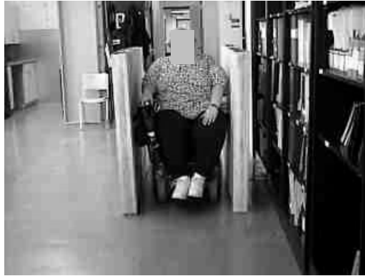
Figure 6 : Level Maneuverability - Straight Wall
