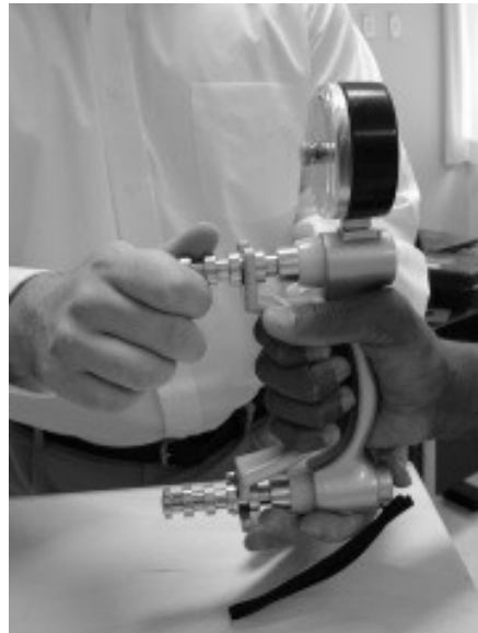
Figure 2 : Measuring grip strength using a grip dynamometer
